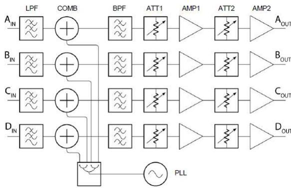
Figure 2: Coupling of pilot-tone inside PT frontend [12].
